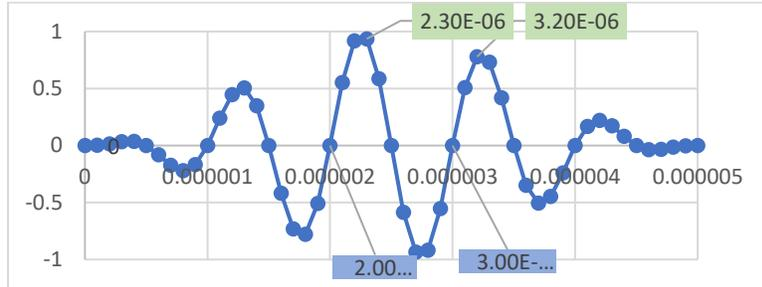
Figure 3: Hanning windowed incident wave signal at  $T = 1 \mu\text{s} \rightarrow f = 1 \text{ MHz}$ .
