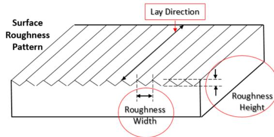
Figure 1: surface characteristics
