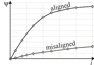
Fig. 3. Magnetisation curves for aligned and misaligned positions.
