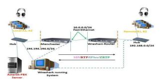
Figure 5 Network Design for VoIP Implementation
